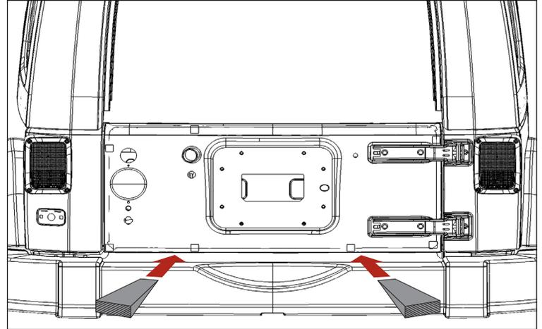
9. Using 13mm socket, remove tailgate hinges from tailgate by removing the 4 bolts indicated on right.
