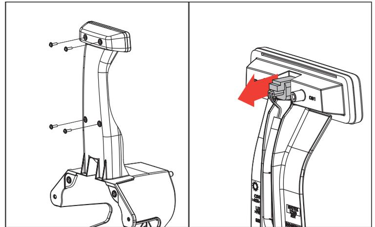
4. Twist and pull rubber bumper to remove from right side of tailgate only.
