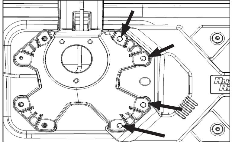
18. Slide spacer plate between tailgate and top left corner of the OE tire carrier. Loosely re-install factory bolts and washers. Repeat for bottom left corner. Some slight shifting of HD Hinge Casting may be required to re-install all 8 tire carrier bolts.
