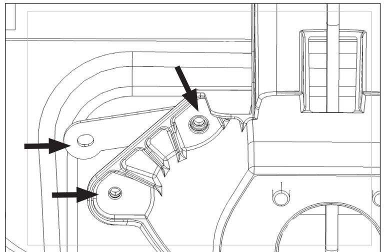
19. Once all bolts are threaded, tighten the 8 bolts around the tire carrier.
