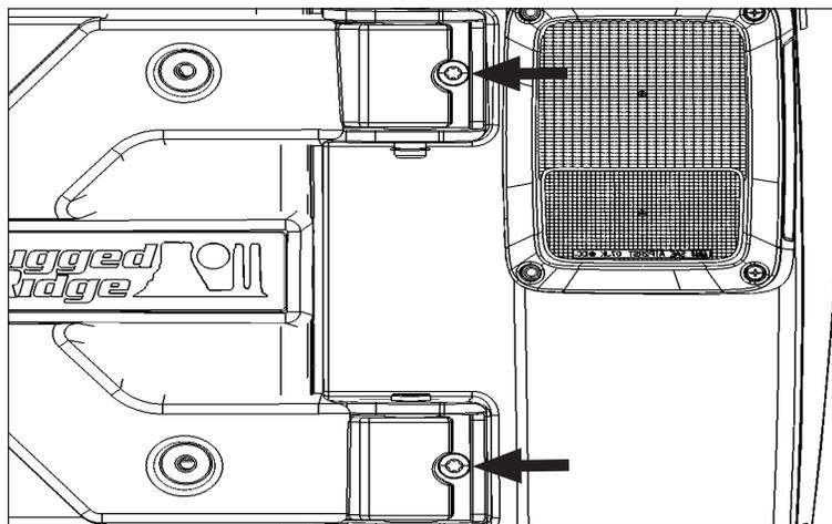
15. Remove the 4 bolts/washers from Step 12. Swing HD Hinge Casting open, making sure not to move the tailgate. Tighten the 4 remaining Torx Head bolts on hinge brackets. Return to closed position.
