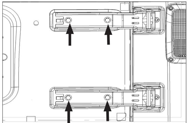
10. Flip hinges to open position. Using a T-50 bit, unscrew stock hinges from vehicle removing the screws indicated at right. This may require using a 10-inch extension with the T-50 bit in order to reach the screws.
