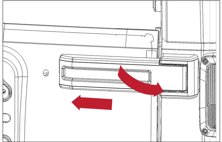
6. Remove plastic clips by pulling lower portion down and away from vehicle.
