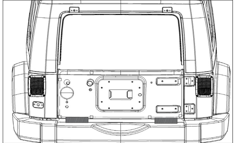
12. Place HD Hinge Casting in position. Reusing 6 factory screws, fasten hinge brackets to vehicle quarter panel. Attach outside screw first, then swing hinge open and install remaining four screws.
