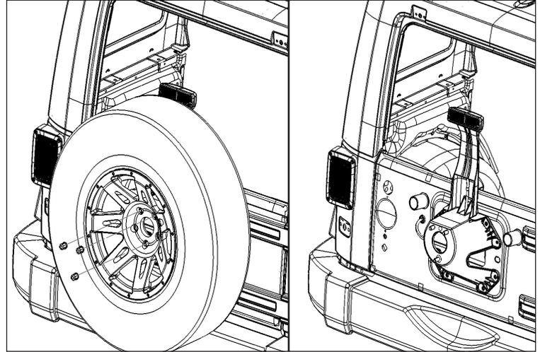
2. Open the tailgate. Using a T-20 Torx bit, remove 4 torx head screws that attach light to factory tire mount. Pull light away from tire mount.
