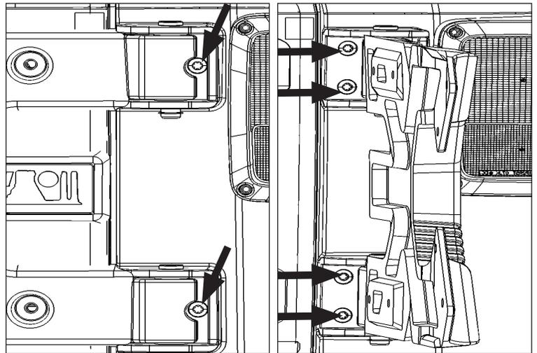
13. Re-using factory bolts and washers removed in step 6, loosely attach right side of HD Hinge Casting.
